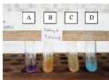
Figure 5. Results of identification of vitamin C with Fehling
